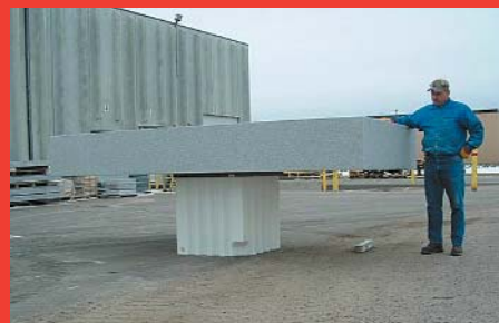
72" x 144" x 18" 18,000 lb. slab of granite setting on empty 120 gallon Tote-A-Lube tank.
